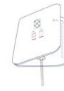
Step4: Peel off the adhesive, and fold the left side over, wait for 15 minutes.
